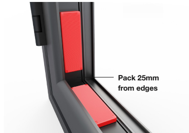
Figure 4.1. Pack 25mm from edges.
